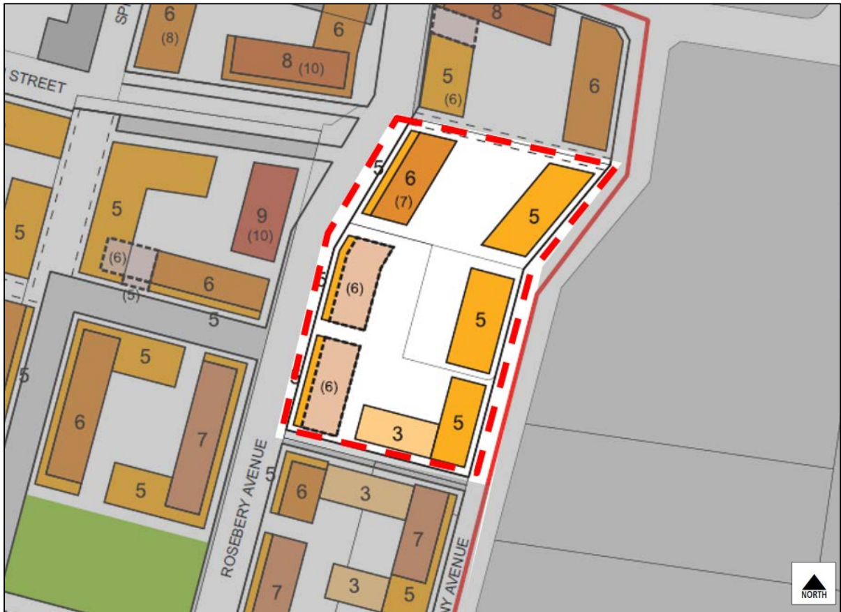
Figure 16: Extract from Sydney DCP 2012 showing current height in storeys control. Brackets indicate the preferred location of any design excellence floorspace which may be awarded.
